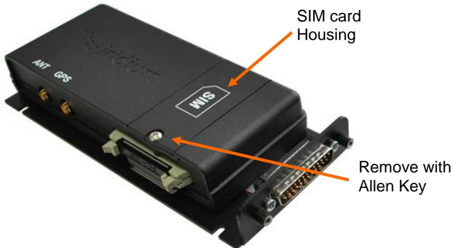
2. Once the cover is removed slide the plastic SIM card holder sleeve (opposite direction of the arrow) to release it from the locked position.
