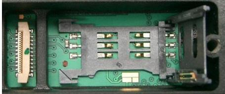
3. Insert the SIM card as shown, with the golden connectors facing inwards and the 'cut corner' of the SIM card facing uppermost.
