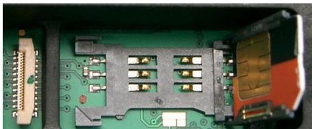
4. Close the plastic sleeve down, and slide in the direction of the arrow until you feel it click into place.
