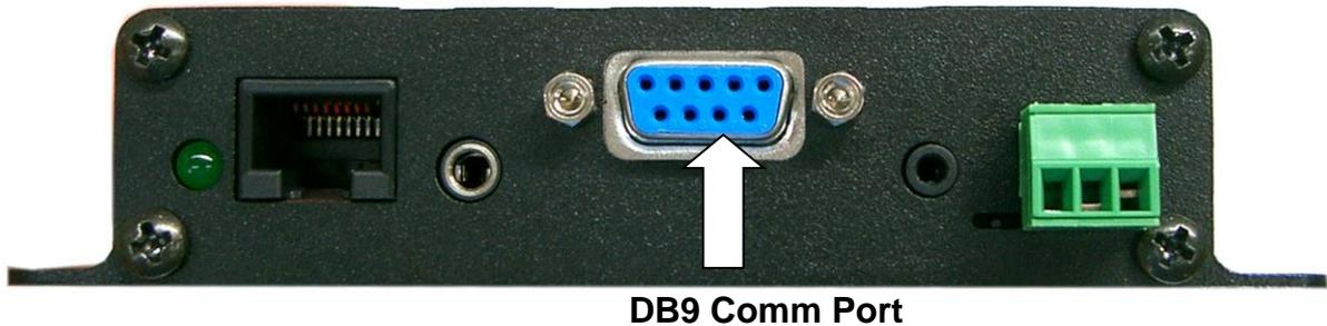
An RS232 serial data port is available via the “Comm Port” allowing data calls, or tracking / alerting modules or a PC to be connected.
