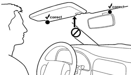
1. Do not place the microphone so that the visor can block it when flipped up or down.
