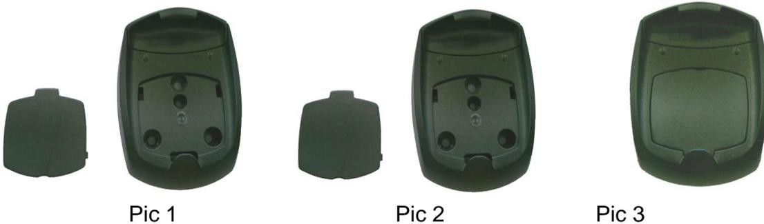
**Step 1** Remove cover on hang-up cup (Pic 1)
