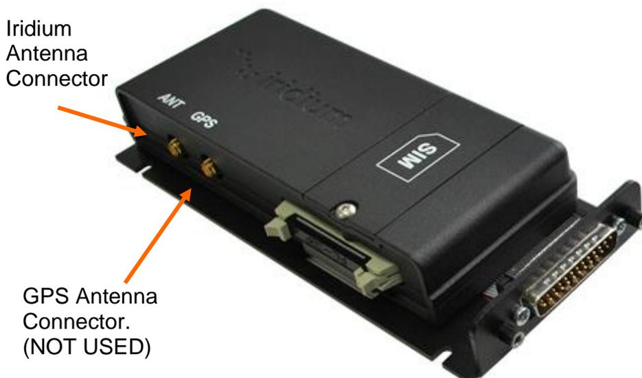
The antenna cable should be connected to the “ANT” antenna socket of the transceiver module as shown above. The transceiver is fitted with an SMA connector, however a converter to change the connector to TNC is included in the kit.
