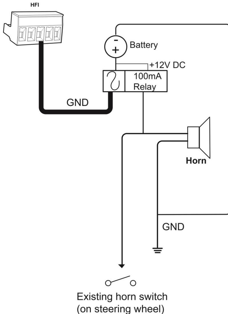
**NOTE:** With this basic configuration, thought needs to be given to the fact that if there is an incoming call while the user is driving, the Horn will subsequently be activated. This may not be a viable option, especially in an urban environment. An alternative configuration would need to be constructed based on the current vehicle configuration, and possibly an additional relay implemented, so that if the ACC are on, the horn won't sound etc.
